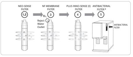
\* The Antibacterial filter contains silver, which is known to inhibit the propagation of microorganisms and to maintain the integrity of the filter.
